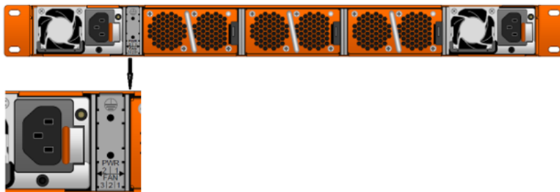
Figure 12 Holes for Ground Screws
